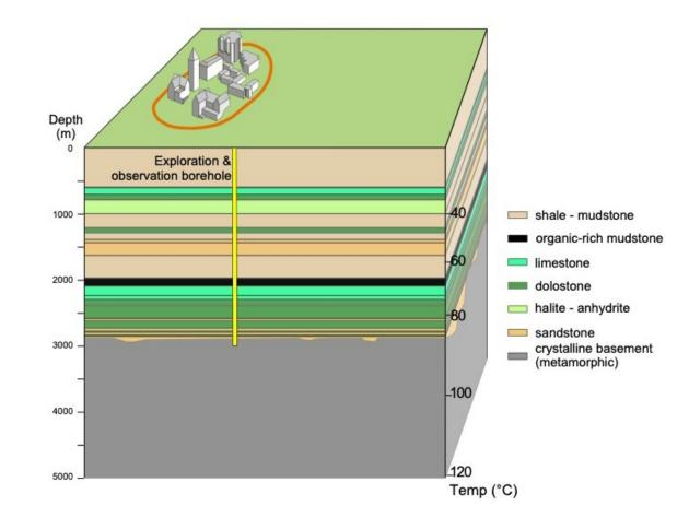
CUBO will Provide Data about Fluids, Stress, Mechanical Conditions, and Temperature
